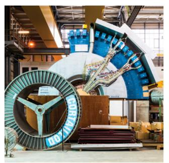
Full-scale wiring test for ATLAS detector
