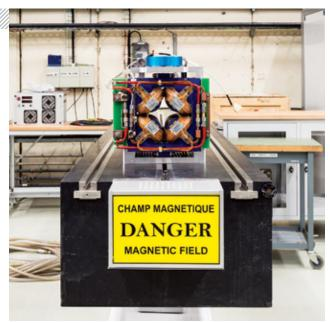
Resistive quadrupole lens for focusing particle beams
